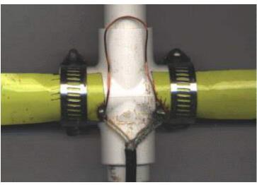
I used 1 1/2 inch hose clamps to attach all the elements on my prototype beam. Others who have duplicated my design have used self tapping screws to attach the elements to the PVC crosses and tees. Performance is the same using either method. The screws are much less expensive but they do not hold the elements as securely. If you do not use 1/2 inch PVC fittings but instead use 3/4 inch, make sure the hose clamps you buy are large enough to fit.
